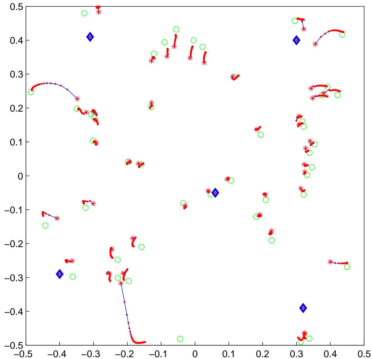
**SDR (ML-SNL formulation), plus a 2nd-stage solution refinement by gradient descent. The distance measurements are noisy.  $\circ$ : true sensor locations;  $\diamond$ : anchor locations;  $*$ : SDR solution;  $—$  : gradient descent trajectory (50 iterations).**
