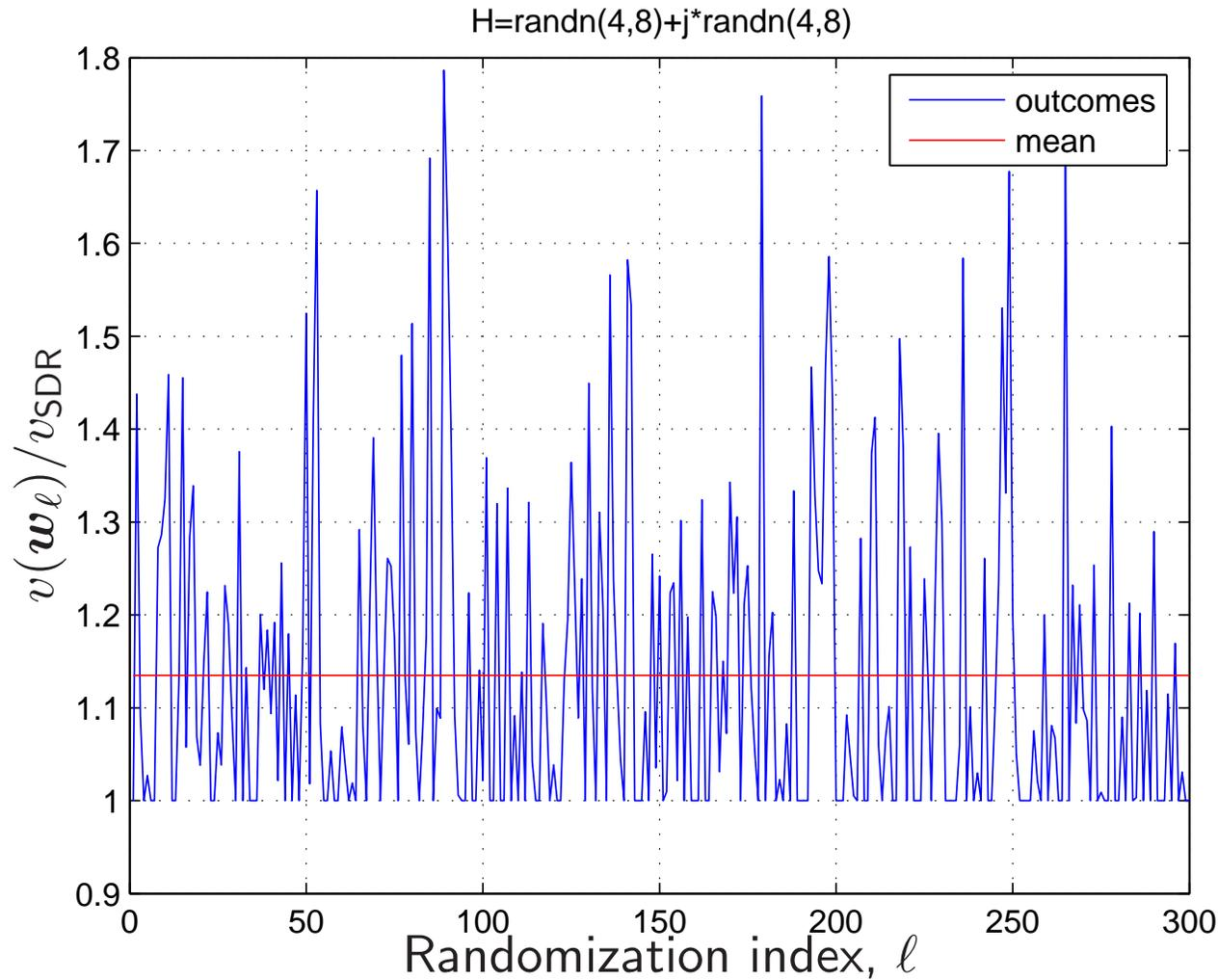
Approximation accuracy of Gaussian randomization in multicast beamforming.  $N_t = 4$ ,  $K = 8$ ,  $v(\mathbf{w}) = \|\mathbf{w}\|^2$  is the objective value,  $v_{\text{SDR}}$  is the optimal value of SDR. Note that for any feasible  $\mathbf{w}$ ,  $v(\mathbf{w})/v_{\text{SDR}} \geq v_{\text{QP}}/v_{\text{SDR}}$  where  $v_{\text{QP}}$  is the optimal value of QCQP. Courtesy to T.-H. Chang and Z.-Q. Luo.
