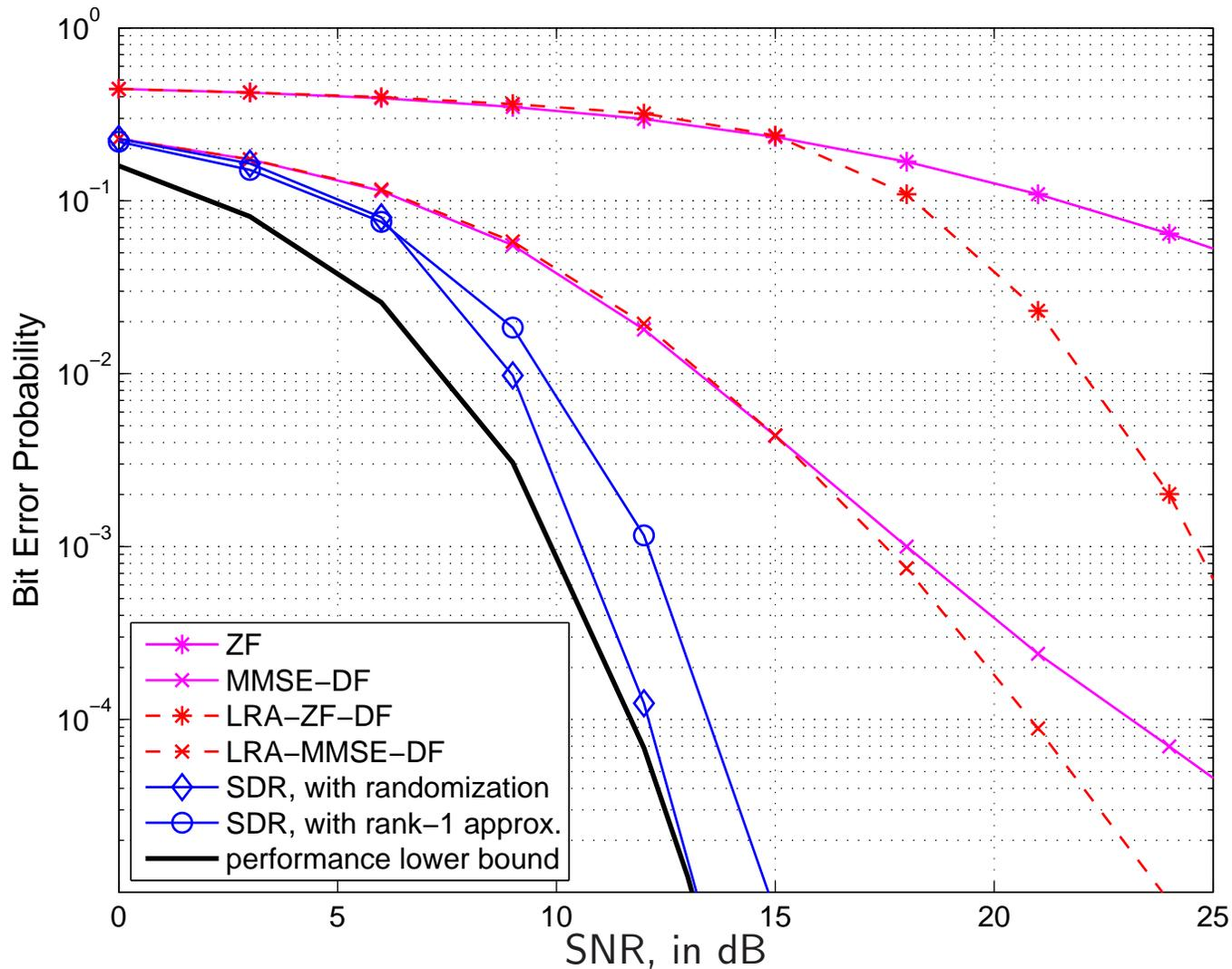
Bit error rate performance under  $(M_r, M_t) = (40, 40)$ . 'ZF'— zero forcing; 'MMSE-DF'— min. mean square error with decision feedback; 'LRA'— lattice reduction aided. 'Randomization' will be explained shortly.
