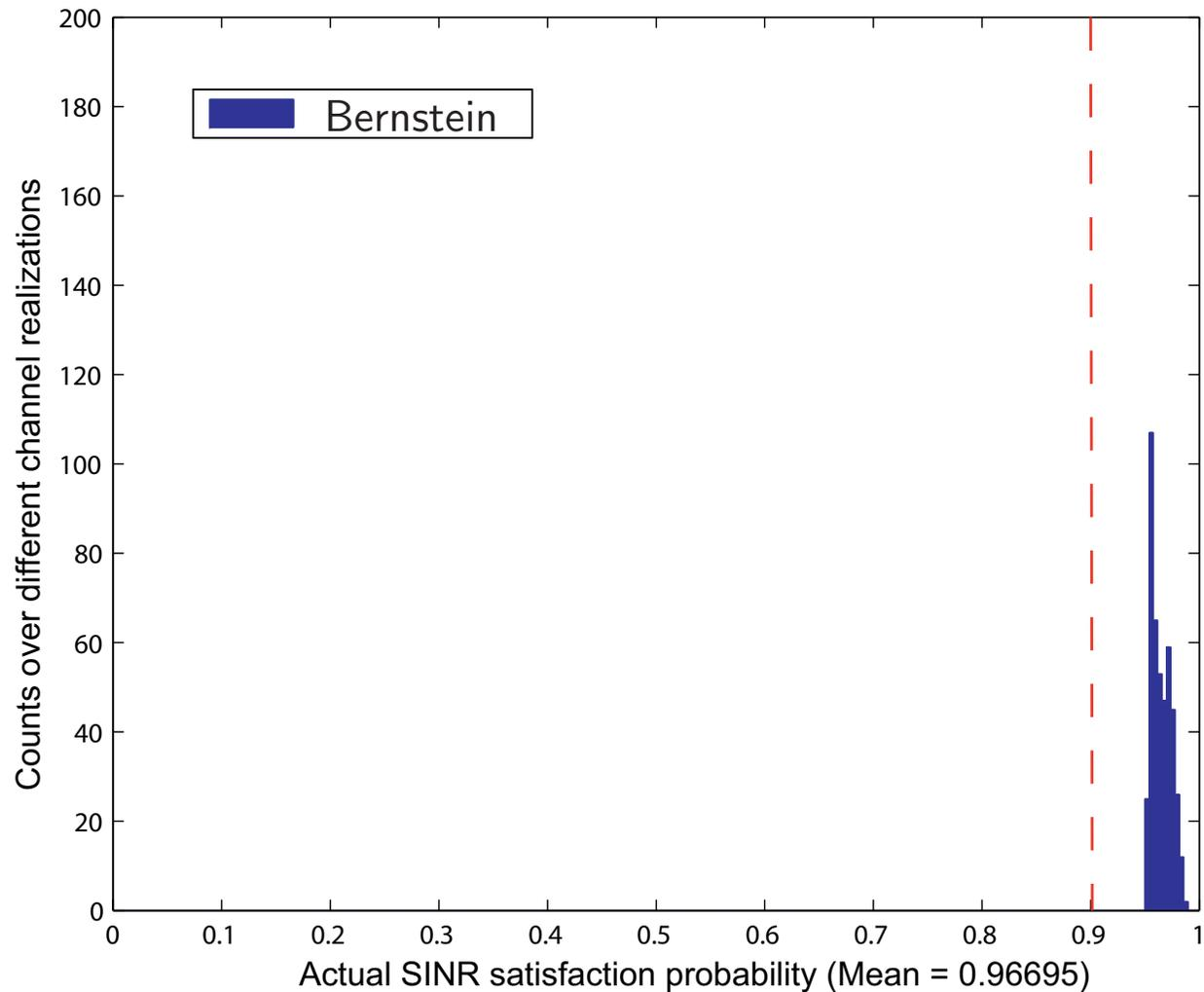
Histogram of the actual SINR satisfaction probabilities of the proposed SDR+Bernstein method.  $N_t = K = 3$ ; i.i.d. complex Gaussian CSI errors with zero mean and variance 0.002;  $\gamma = 11\text{dB}$ ;  $\rho = 0.1$  (90% SINR satisfaction).
