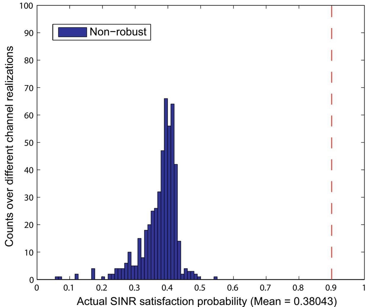
Histogram of the actual SINR satisfaction probabilities of the non-robust QoS-assured design.  $N_t = K = 3$ ; i.i.d. complex Gaussian CSI errors with zero mean and variance 0.002;  $\gamma = 11\text{dB}$ . The design has more than 50% outage most of the time.
