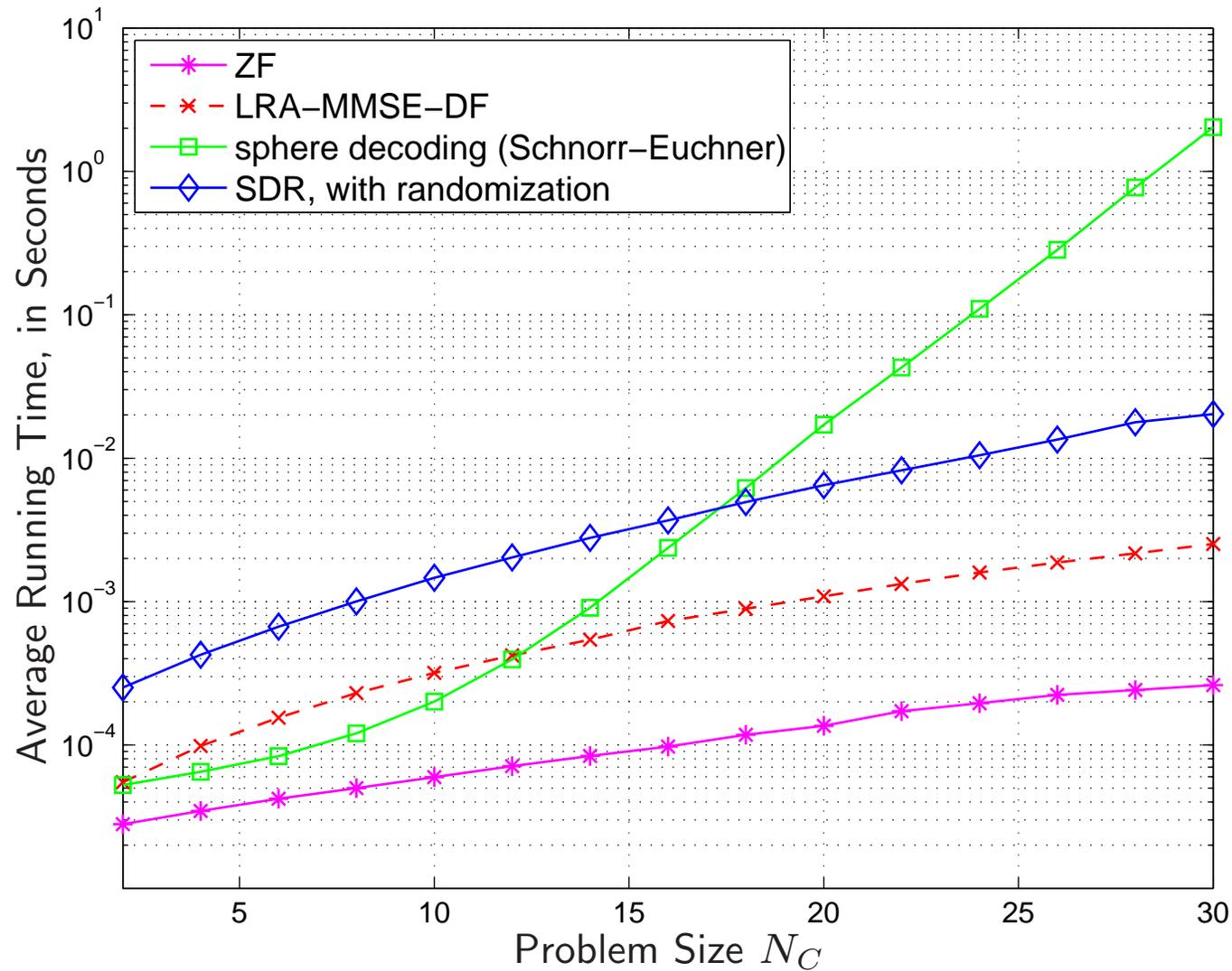
Complexity comparison of various MIMO detectors. SNR= 12dB. Sphere decoding is an exact ML method.
